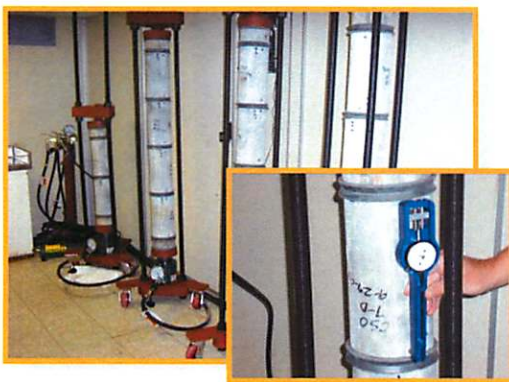
CREEP-LOAD TEST - HIGH STRESS CONCRETE
