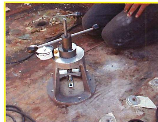
ROOFING FASTENER PULLOUT TEST UCSD HOSPITAL CENTRAL PLANT
